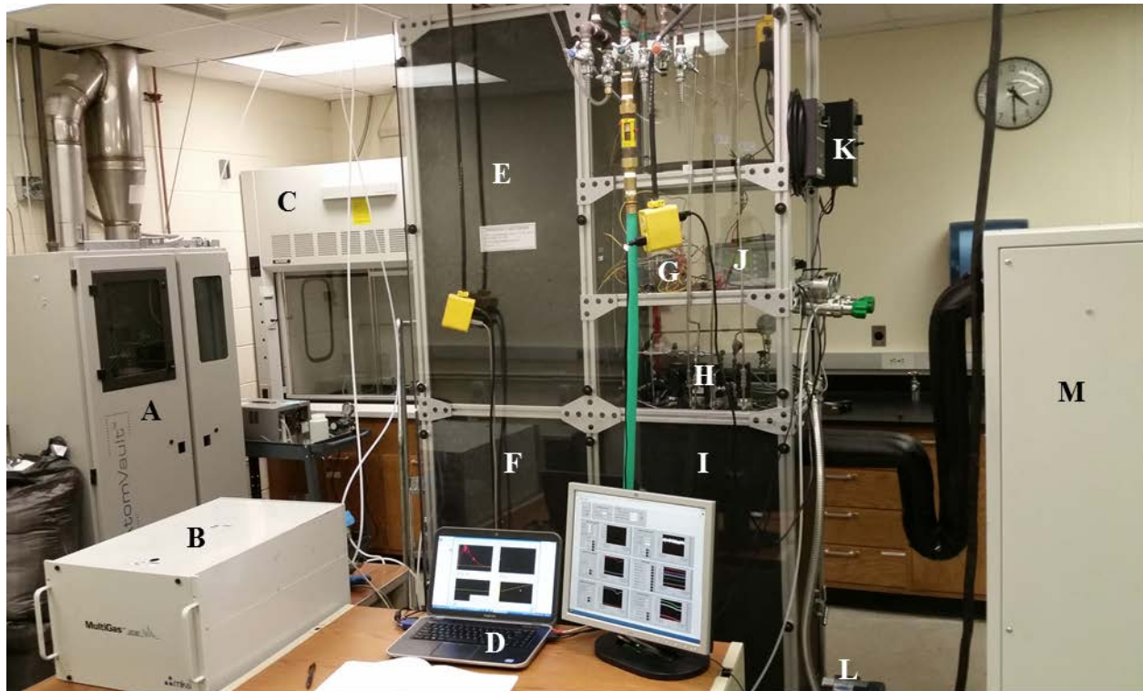
Figure 4-6 Natural gas capable apparatus with cylinder gas cabinet (A), FTIR (B), exhaust fume hood for flaring and venting (C), computer control interface (D), bubbler and separator cold box (E), reservoir cold box (F), data acquisition (G), mass flow controllers (H), heat exchange and pumping cold box (I), mass flow controller power supply (J), pump motor controller (K), pump motor (L), cryocooler (M)
