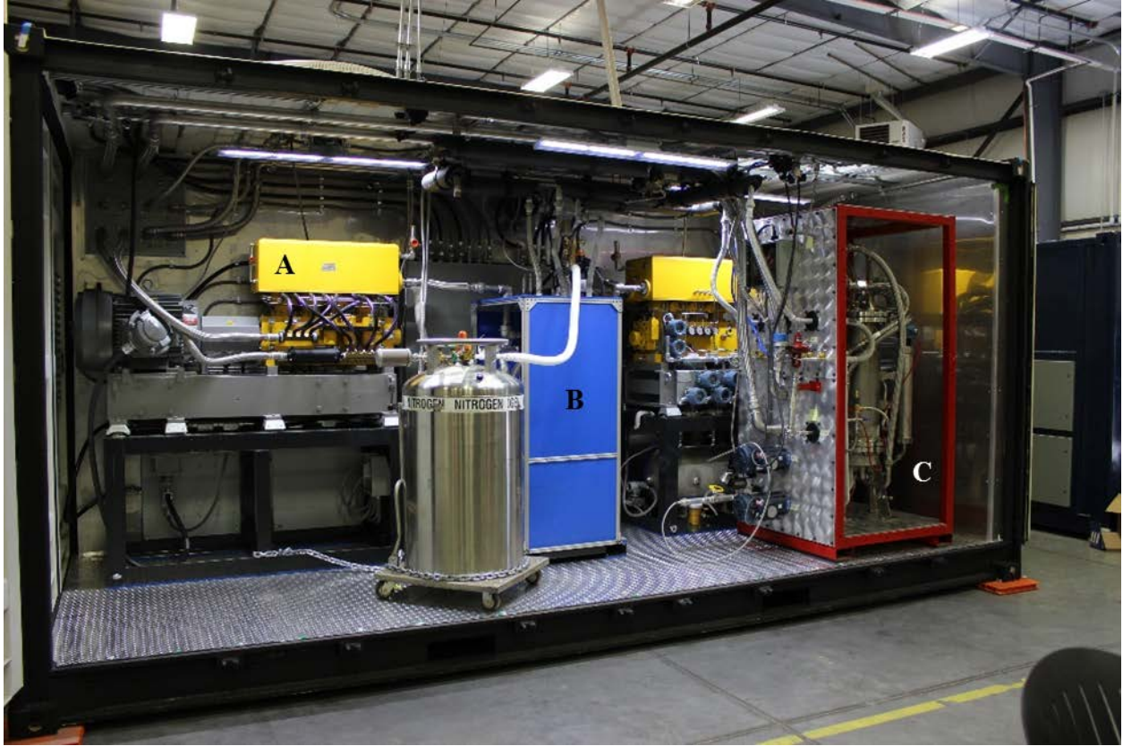
Figure 4-5 CCC skid for CCC ES with cryogenerators (A), contact liquid cooling (B), and bubbling CO 2 desublimating column (C)
